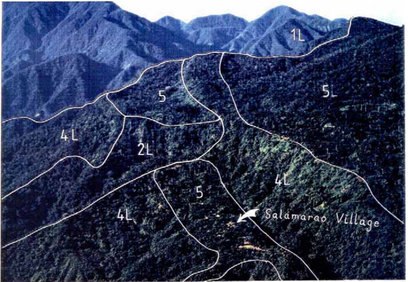
Figure 6. Landslide hazard in upper Nggurambusu watershed in vicinity of Salamarao. 1L Very high landslide hazard; 2L High landslide hazard; 4L Low landslide hazard; 5 Safe. Shifting cultivation occurs on most areas mapped as 4L. These areas are subject to infrequent shallow landslides. "Safe" areas illustrated here are limestone-capped dip slopes. These areas are generally the safest sites in the mountains and most villages are located in them.
