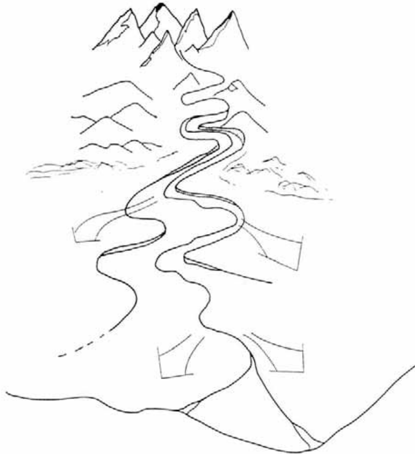
Figure 11. Schematic diagram of major river courses on Guadalcanal Plain. In large floods, overflows generally occur at the head of the Plains and on the deltas near the coast. At these locations the confining terraces are relatively low. Terraces tend to be higher in the middle sections of the rivers.
